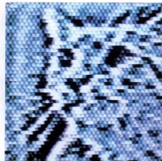
Silicon sees a cat. This retina-on-a-chip mimics the functions of cells in the human eye.
